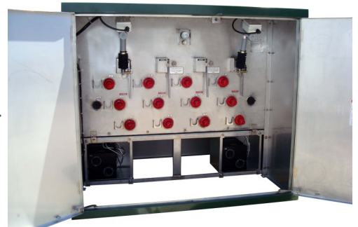
Trayer 800 series Solid Dielectric Load Break Switch 25kV, 600A, 4 ways, 4 ways switched Padmount Vacuum Load Break Switch
