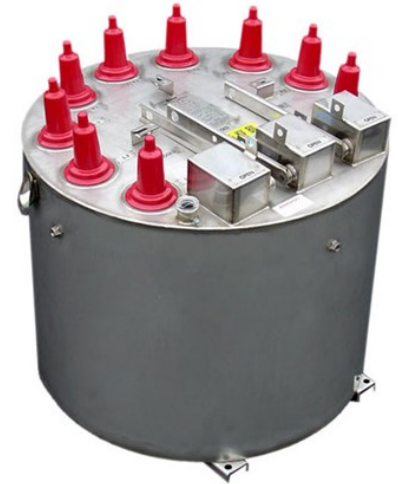
Trayer 100 series Solid Dielectric Load Break Switch 25kV, 600A, 3 ways, 3 ways switched Submersible Vacuum Load Break Switch
