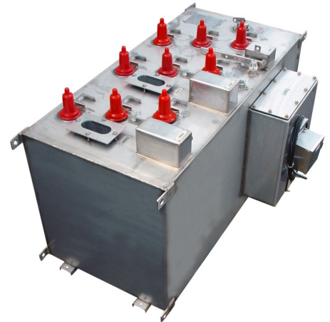
Trayer 3100 series Solid Dielectric Load Break Switch 25kV, 600A, 3 ways, 2ways switched 1 way protected Submersible Vacuum Fault Interrupter
